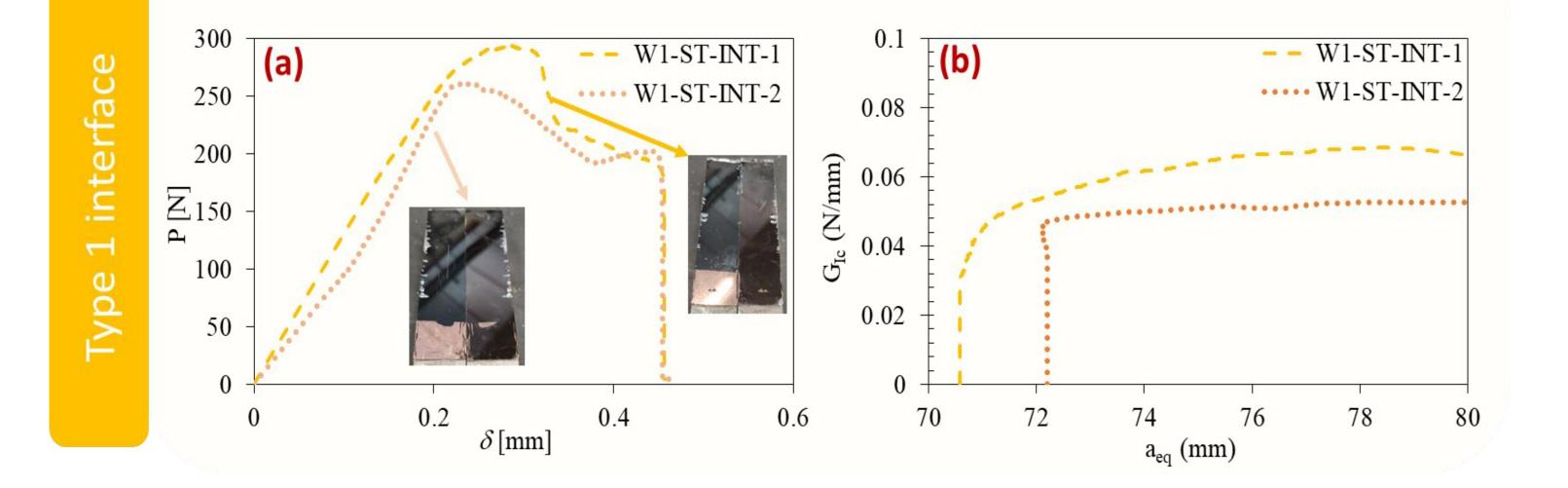
**Figure 3**. Type 1 interface quasi-static results. (a) Load-displacement curve. (b) Rcurve.
