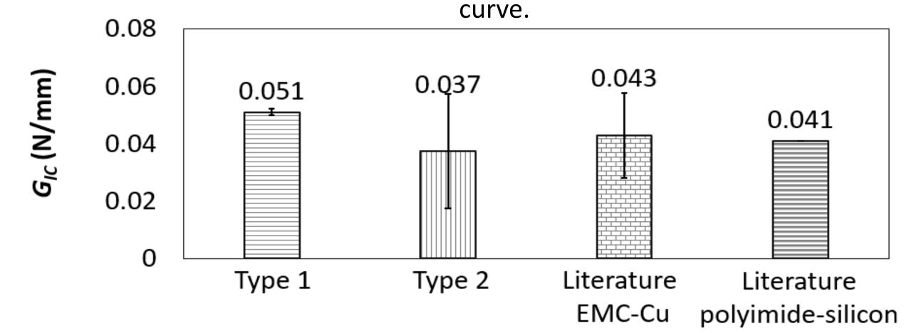
We performed Double Cantilever Beam (DCB) experiments on two different Silicon wafers as shown in Figures 1 (Dimensions in mm) and 2. The material properties of both tested material and the adhesive used for DCB sample preparation are listed in Tables 1 and 2.
