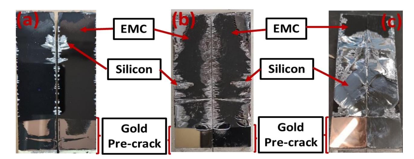
**Figure 6**. Typical fracture surfaces. (a) Interfacial failure. (b) Mixed failure. (c) Silicon failure.
